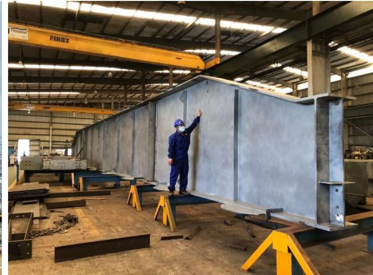
24m crane beam under fabrication
