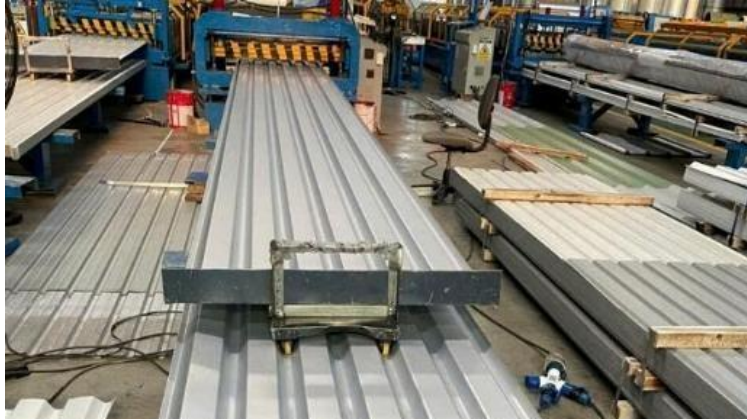
02-C Sheeting Forming Roll-forming for roof and wall cladding sheets
