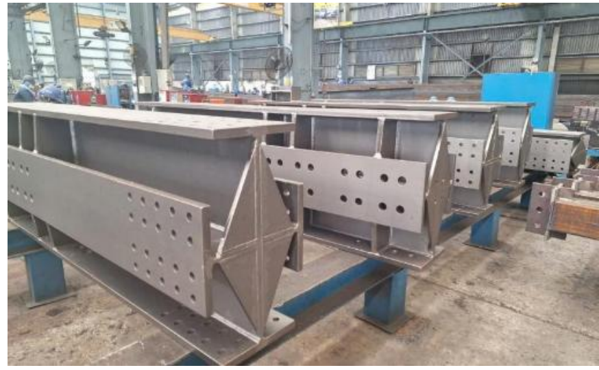
07.C Finishing Product – Star Column Steel star-shaped column completed for delivery
