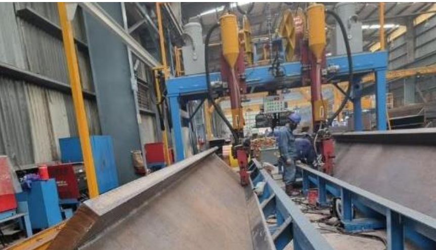
03-B Auto Welding Gantry Maximum web width: more than 1500 mm Maximum flange width: more than 500 mm
