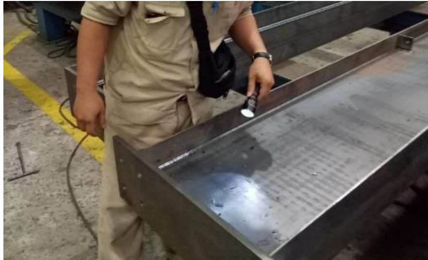
06-A Welding Inspection – Initial Inspection Initial inspection for visual welding quality and dimensions
