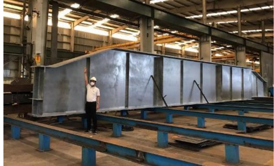
07.A Finishing Product – Big Beam Final assembled and painted main beams
