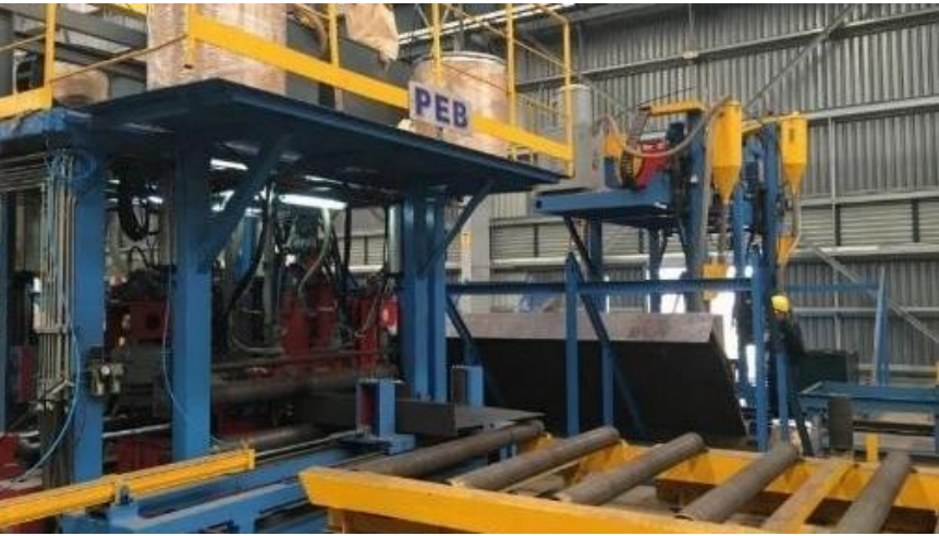
03-A Auto Welding SAW (Pull-through) Maximum web width: up to 1500 mm Maximum flange width: up to 500 mm
