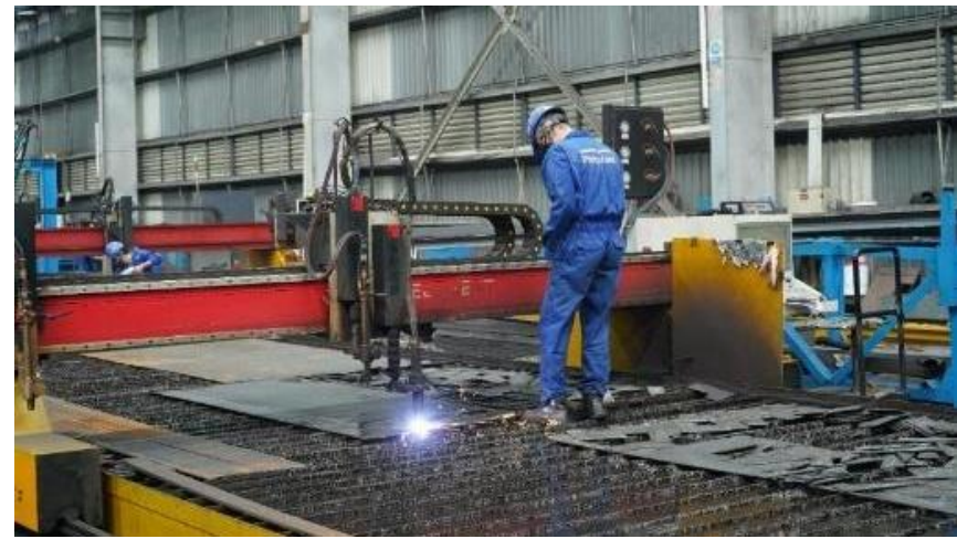
02-C Plasma Cutting Machine For cutting intricate and detailed components Use for: metal sheets, complex shapes, and fine-detail parts
