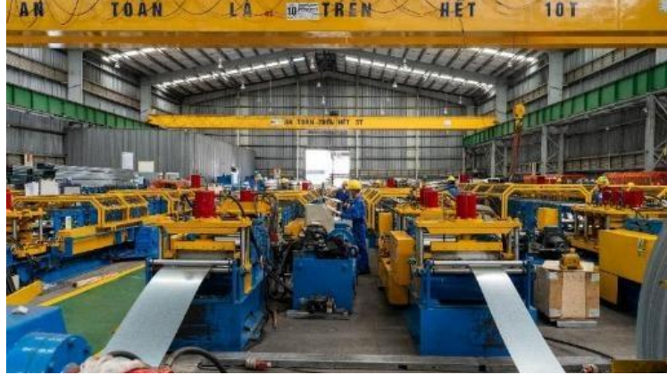
02-A Purlin Forming Cold-formed purlins for roof and wall support systems
