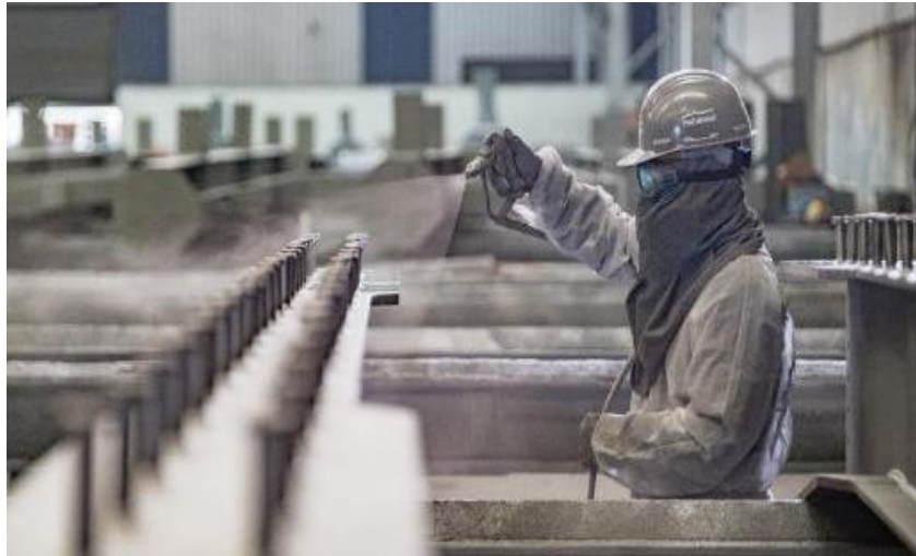
09 Painting Protective coating application for corrosion resistance
