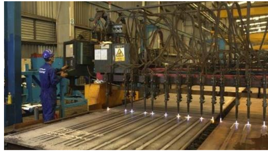
02-B CNC Cutting Machine Maximum thickness: up to 80 mm Length capacity: 12 meters High precision cutting
