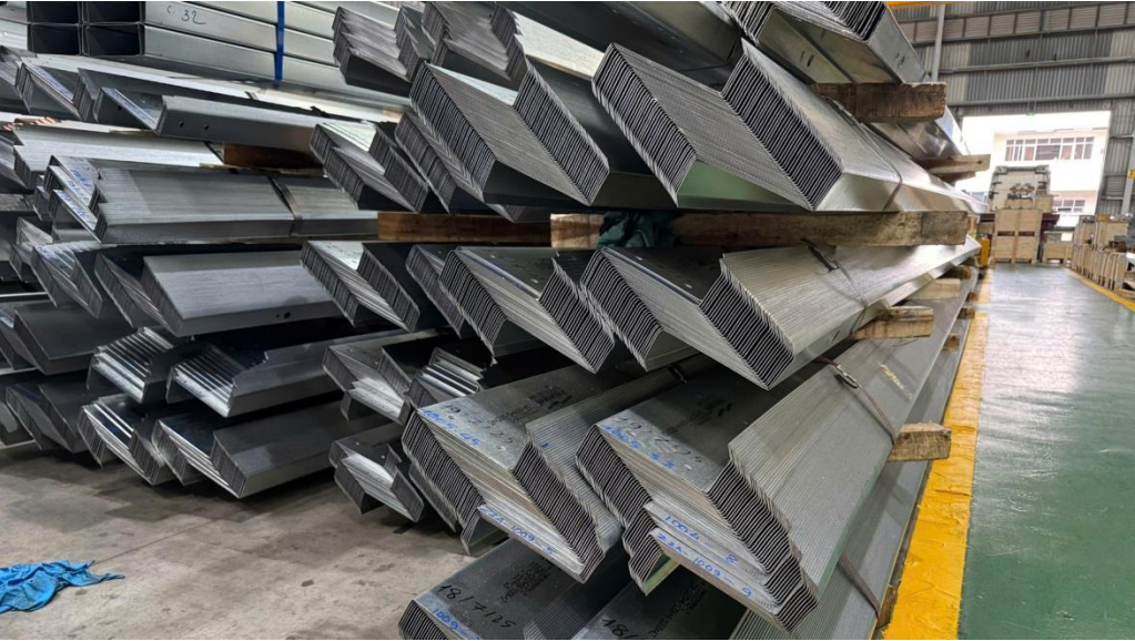
03-A Packing of Purlins for Delivery Pre-arranged bundles for efficient loading and protection
