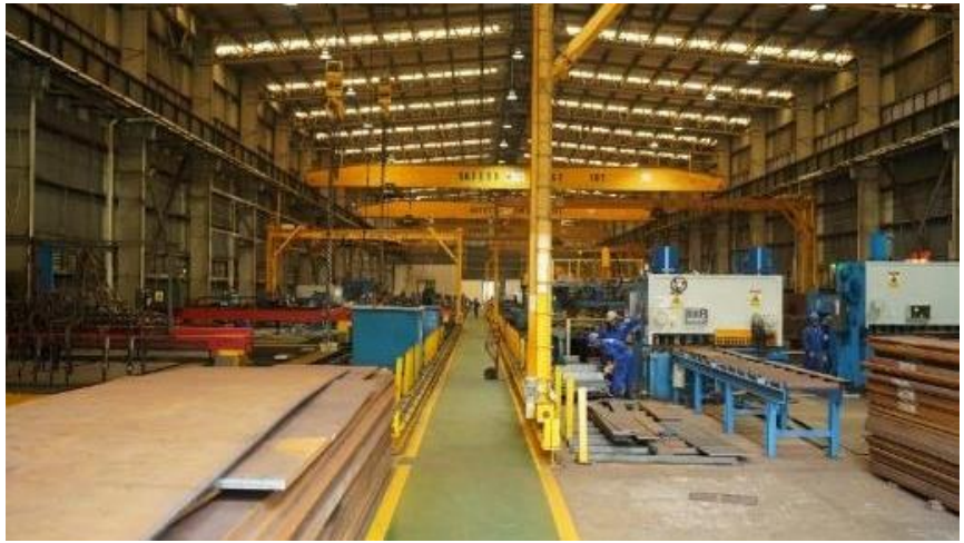
02-A Shearing Machine Maximum thickness: up to 12 mm Length capacity: 6 meters
