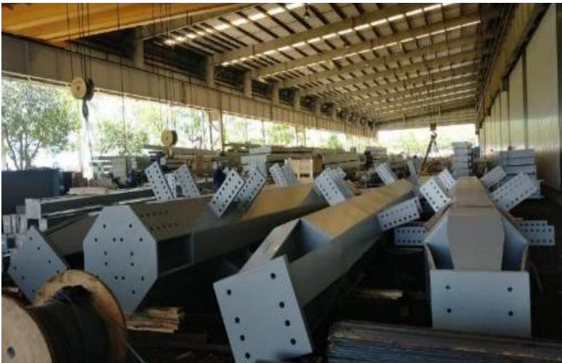
10 Finishing Product – Box Column Completed box columns, ready for delivery or assembly
